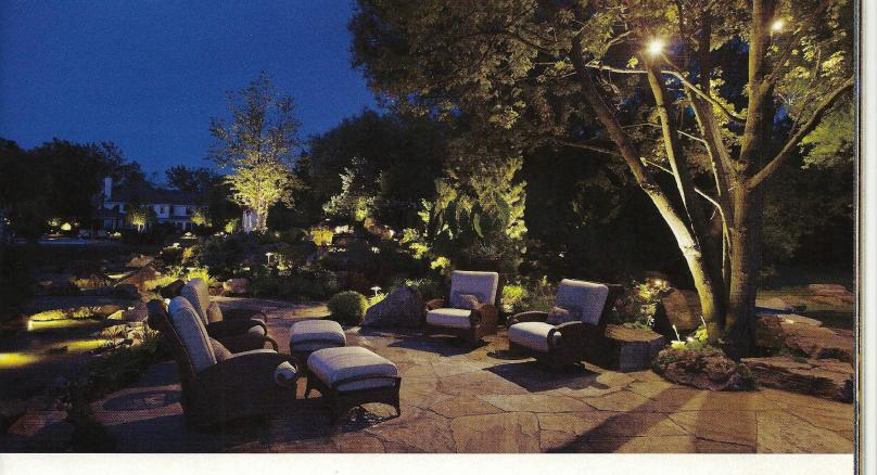
**Above:** Workers wired an existing patch of maple trees with 8.5-watt, 60-degree LED directional spot down lights. They mounted the lights 25 feet up from the ground, and secured the light to the tree with a tree-mount bracket with tree-safe stainless steel screws.
